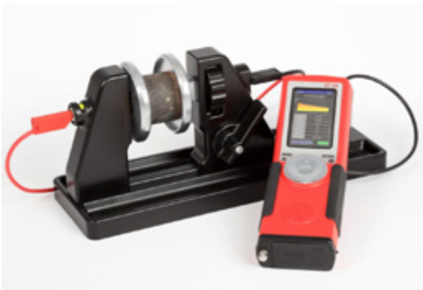
IP/Resistivity Module with Small Sample Holder
