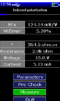
IP/Resistivity Measurement IP Decay Curve
