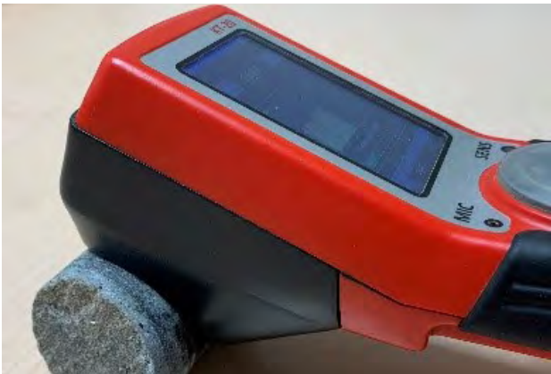
Curved Sensor Measuring Core Sample
