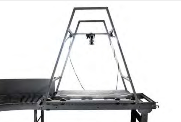
Roller racking camera frame with wheels
