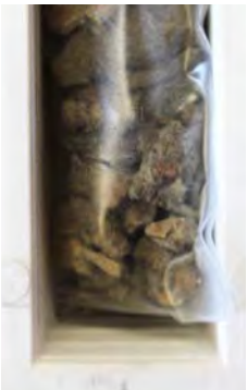
Heat-sealed layflat tube in plastic core tray
