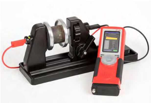
IP/Resistivity Module with Small Sample Holder
